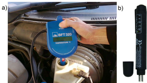
Fig. 1 a) The brake fluid tester BFT 320 during the measurement, b) 4-diode tester
