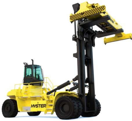
Fig. 2 Container stacker with front sided lift. Source: www.directindustry.com
