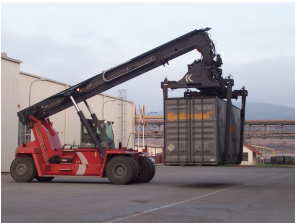
Fig. 3 Reach stacker with special attachment for handling of the ITU (DB Megabox), Source: authors
