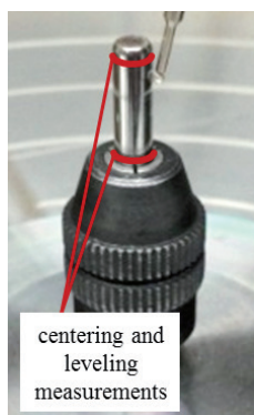
Fig. 11 Centering and leveling planes in unworn areas of the pin
