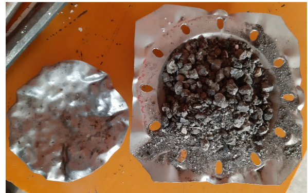
Fig. 12 Panel with core made of resin and pumice after testing
