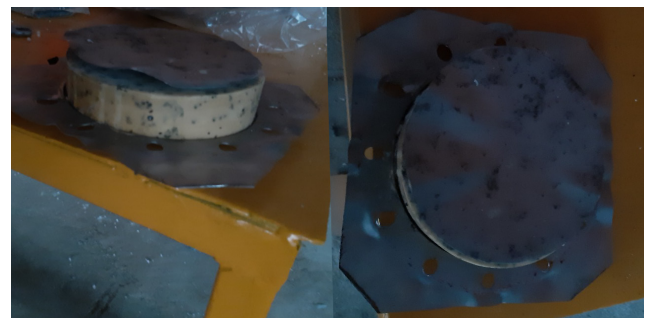
Fig. 13 Panel with core made of foam and pumice after experiment
