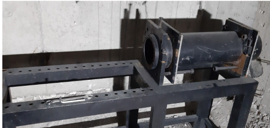
Fig. 9 Shock tube used in the experimental test
