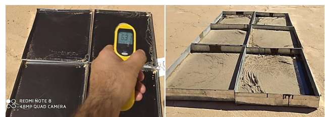
Fig. 1 Bitumen before and after aging
