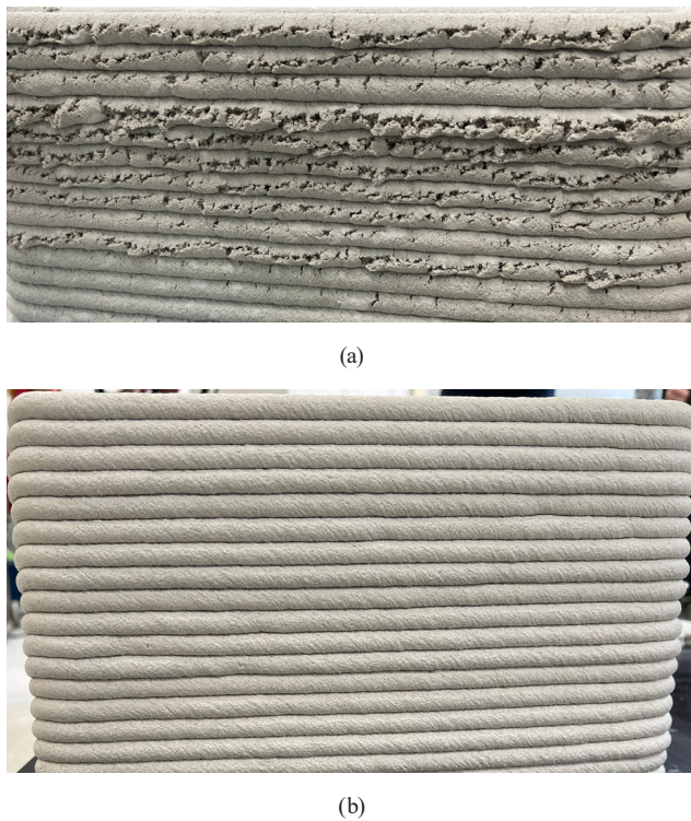
Fig. 11 Quality of the printed walls; (a) w/d = 0.140 ; (b) w/d = 0.145
