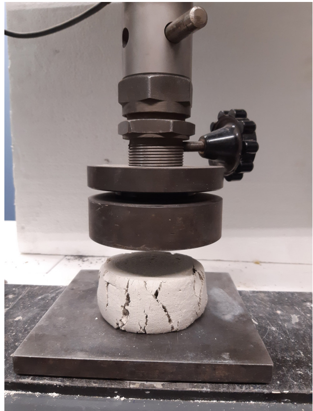
Fig. 4 Green strength test setup
