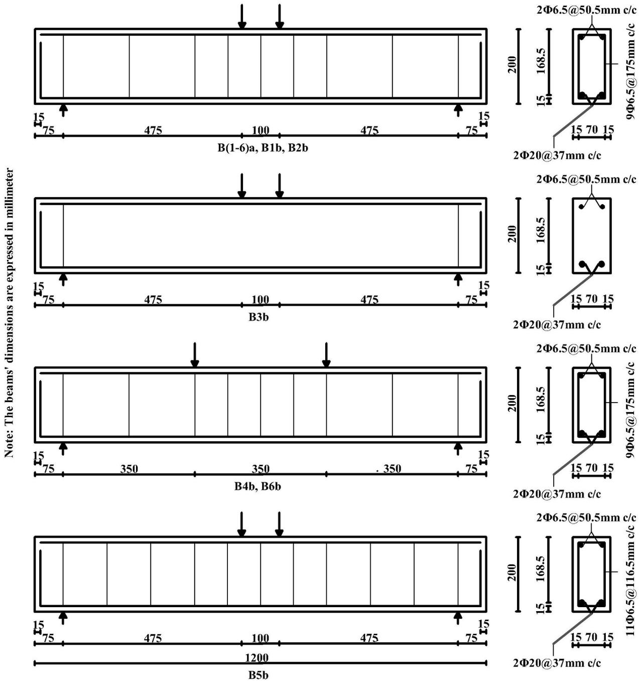
Fig. 1 UHPFRC-CA beam's longitudinal-cross section
