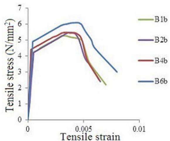
Fig. 6 Tensile stress-strain of the UHPFRC-CAs/UHPFRC
