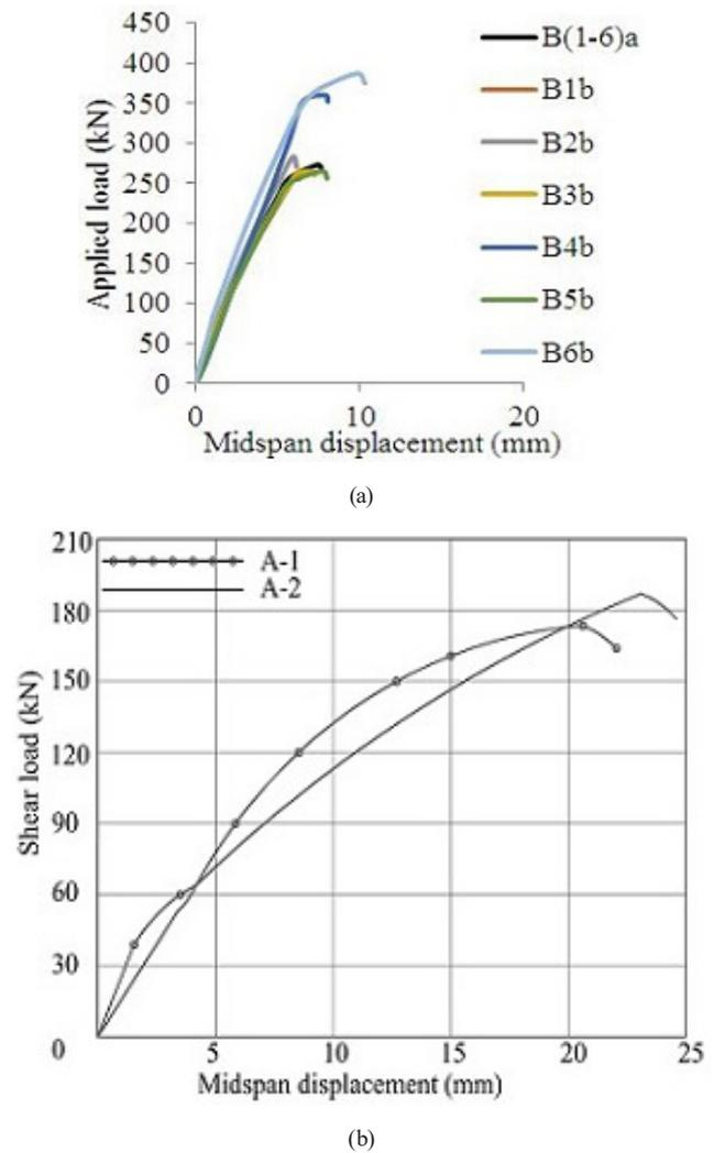
Fig. 5 Load-midspan displacements of the beams: (a) UHPFRC-CA beams, (b) Ahmad et al.'s [18] beam
