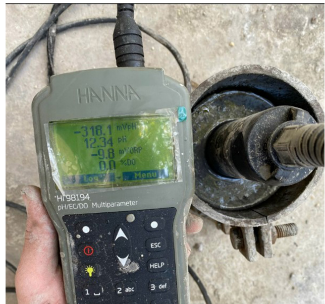
Fig. 2 The pH measurement of fresh concrete mixtures
