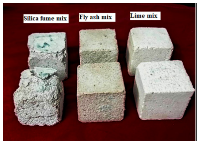
Fig. 7 The studied mortars after the artificial ageing
