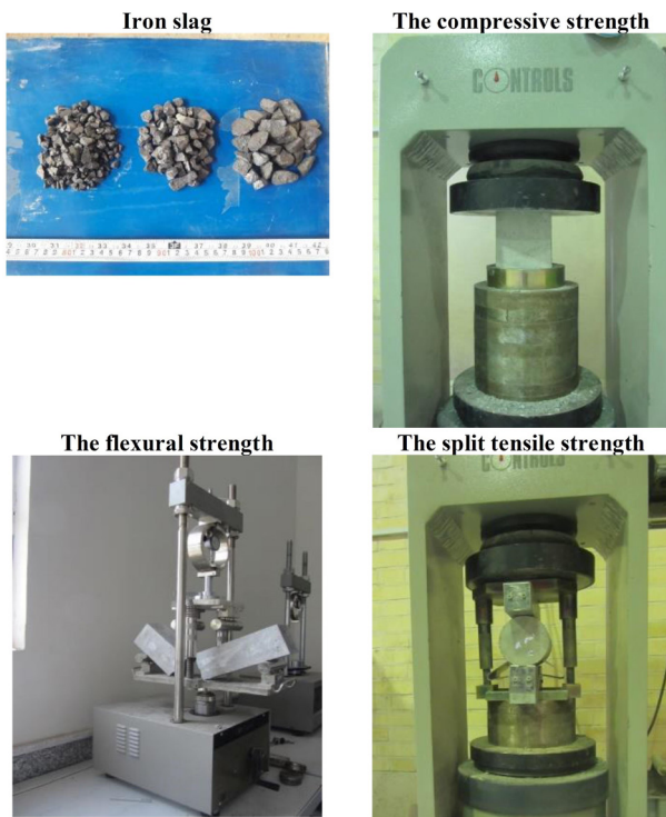
Fig. 2 Iron slag and the strength tests
