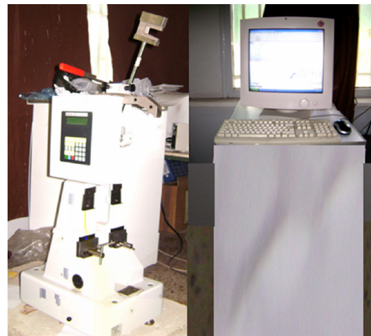
Fig. 3 Zwick/Roell type Charpy impact machine used
