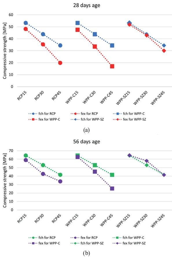
Fig. 7 Comparison of theoretical compressive strength for cement hydration (*fch*) and experimental results (*fex*) for the mortar samples using RCP, WPP-C and WPP-SZ for a. 28 days and b. 56 days age
