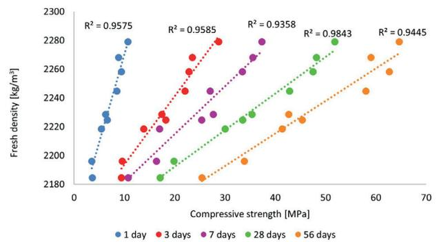
Fig. 11 Correlation between the fresh density of investigated mortar samples and compressive strength
