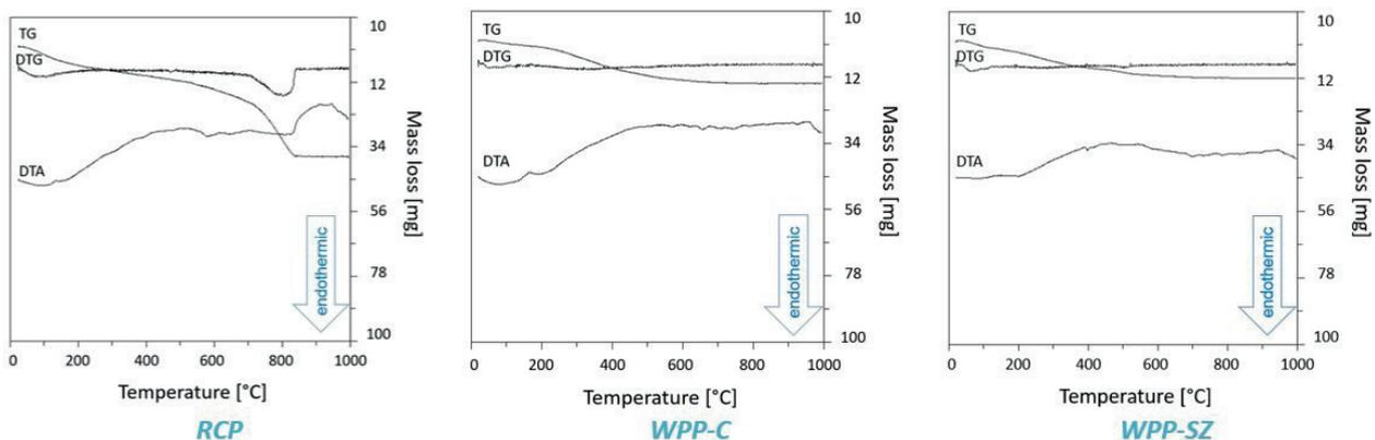
Fig. 3 TG/DTG/DTA curves of RCP, WPP-C and WPP-SZ
