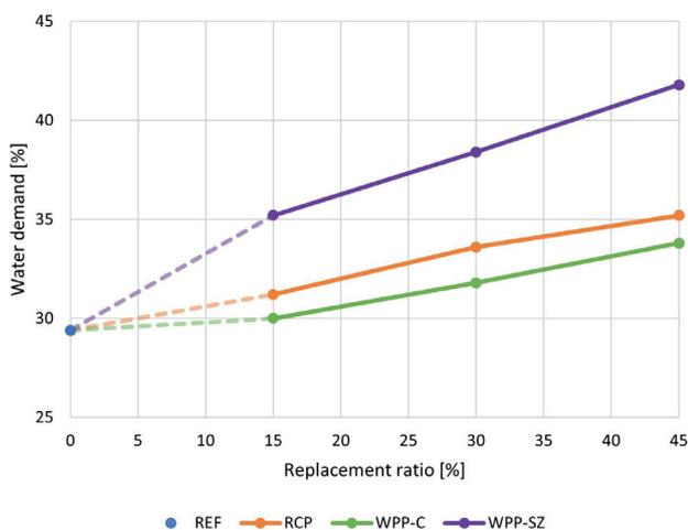
Fig. 13 Water demand of the blended cement pastes utilizing RCP, WPP-C and WPP-SZ
