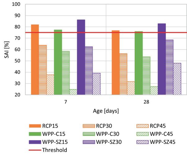
Fig. 8 Comparison of SAI for blended types of cement with the requirement of ASTM C 618
