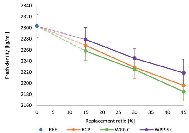
Fig. 10 Fresh density of mortar samples incorporating RCP, WPP-C and WPP-SZ
