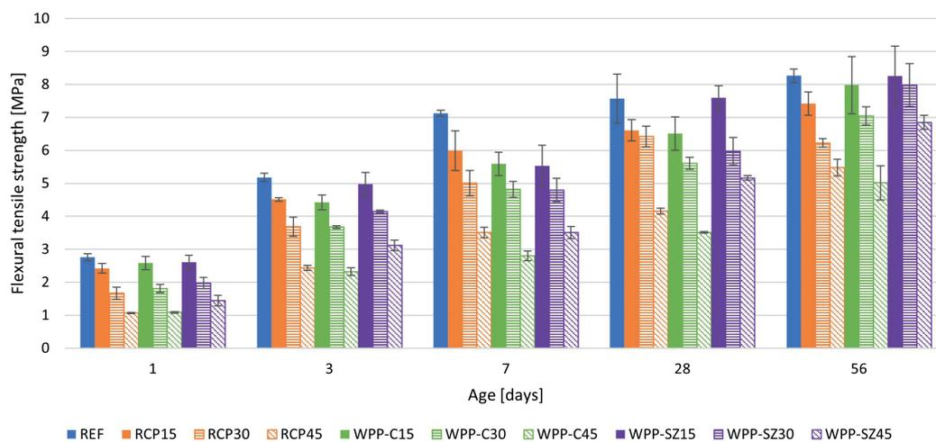
Fig. 5 Flexural tensile strength results of the mortar samples incorporating RCP, WPP-C or WPP-SZ
