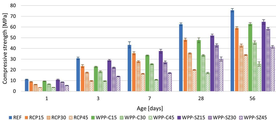
Fig. 6 Compressive strength results of the mortar samples incorporating RCP, WPP-C or WPP-SZ
