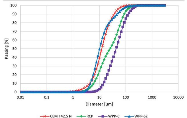
**Fig. 1** Grading curve for the cement, RCP and WPPs
