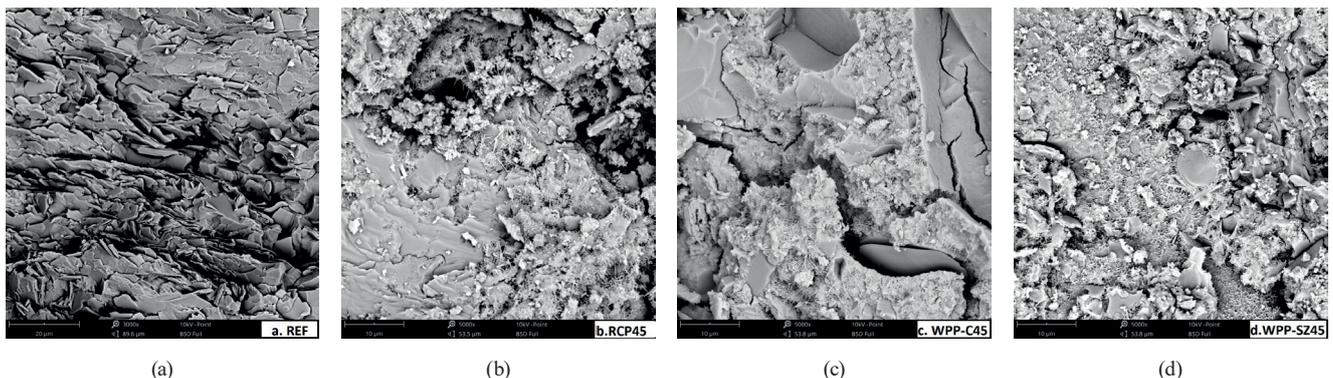
Fig. 9 SEM analysis of reference mortar (a) and mortars incorporating 45% substitution by RCP (b), WPP-C (c) and WPP-SZ (d)
