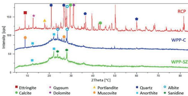
Fig. 4 X-ray diffraction patterns of RCP, WPP-C and WPP-SZ
