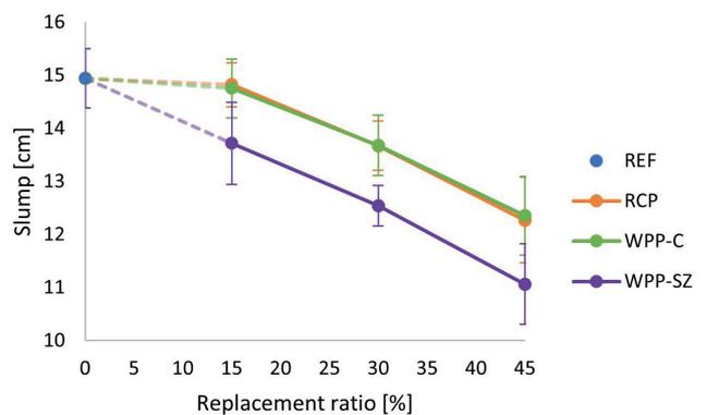
Fig. 12 Slump values of the mortar samples with RCP, WPP-C and WPP-SZ
