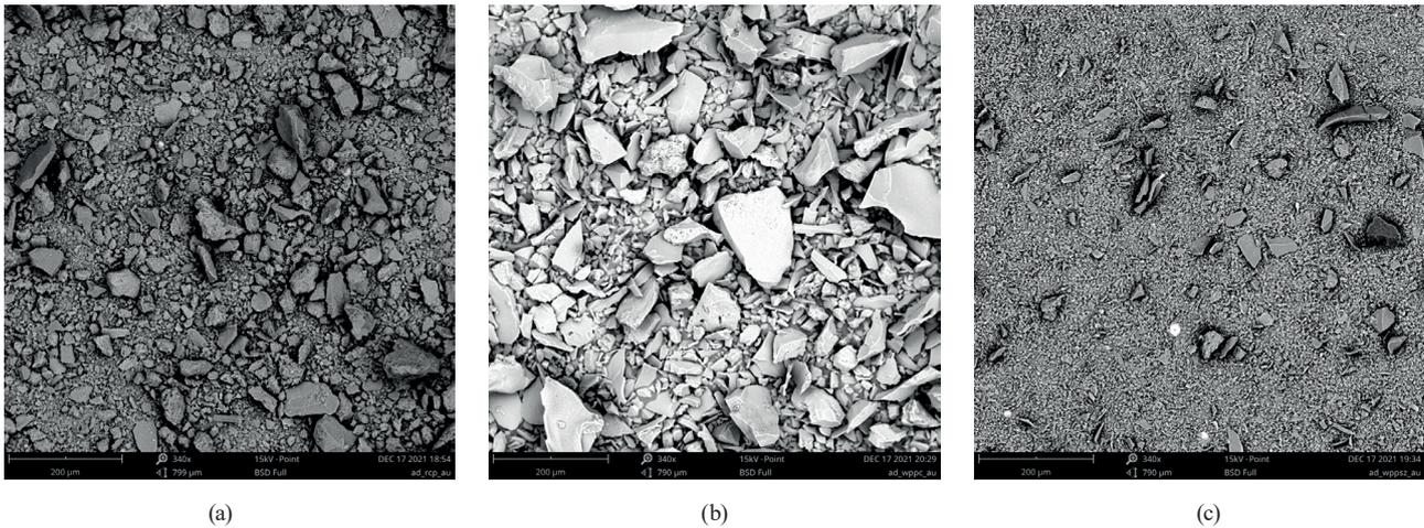
Fig. 2 SEM images of (a) RCP, (b) WPP-C and (c) WPP-SZ
