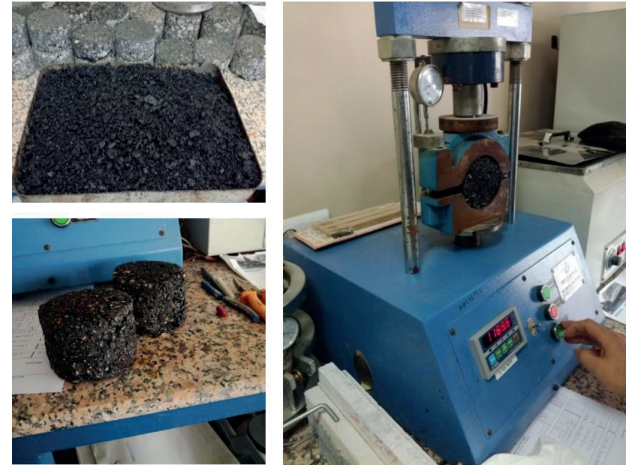
Fig. 3 Asphalt concrete sample preparation and Marshall Stability Test
