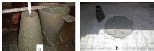
Fig. 7 Workability tests of (a) Normal Concrete and (b) ECC concrete
