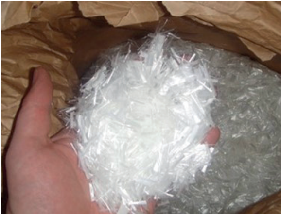
Fig. 1 Polyvinyl alcohol (PVA) fibers from Kurary Japan, used in ECC
