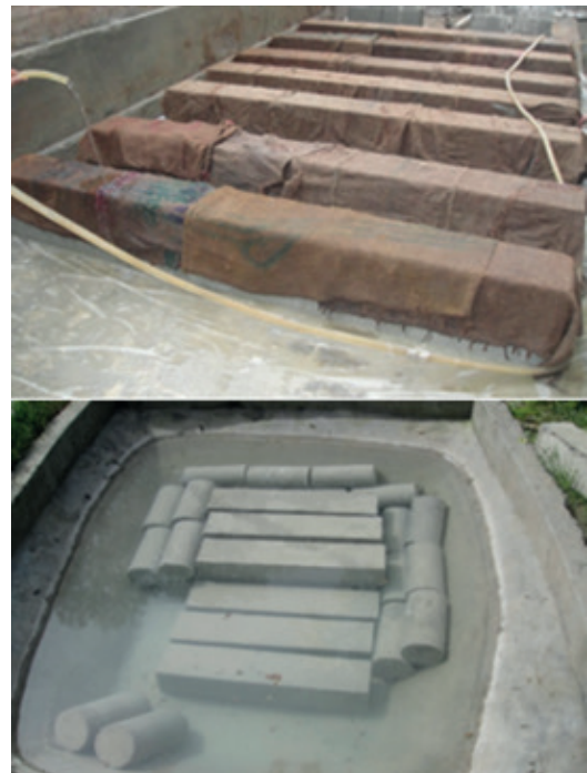
Fig. 5 Curing of full-scale beams, cylinders, and small beam specimens
