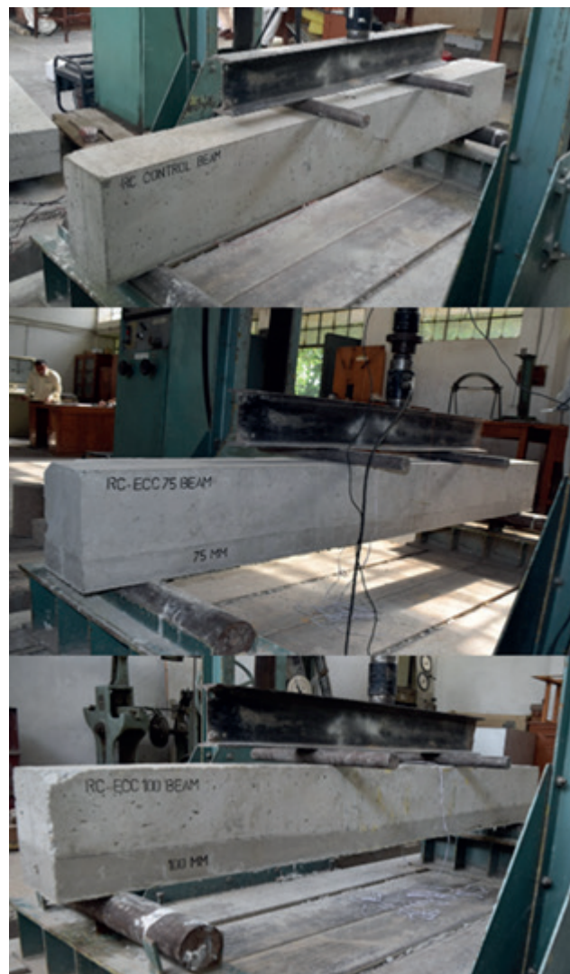
Fig. 8 Testing of the full-scale beam in straining frame under third point bending [38]
