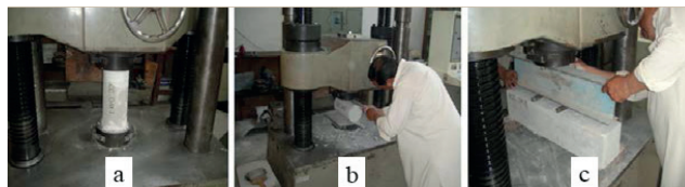
Fig. 6 Visuals of the tests for determination of the mechanical properties: (a) Compressive (b) Split tensile and (c) Flexural strengths of both control concrete and ECC
