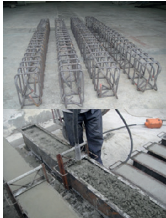
Fig. 4 Casting of full-scale beam specimens
