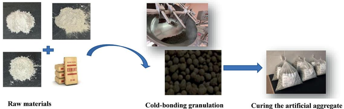
Fig. 2 Cold-bonding manufacturing process
