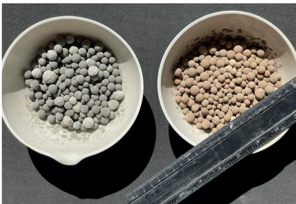
Fig. 5 Effect of sintering on the color and shape of artificial aggregates, (left) is cold-bonded FA artificial aggregate, and (right) is sintered FA artificial aggregate at 900 °C
