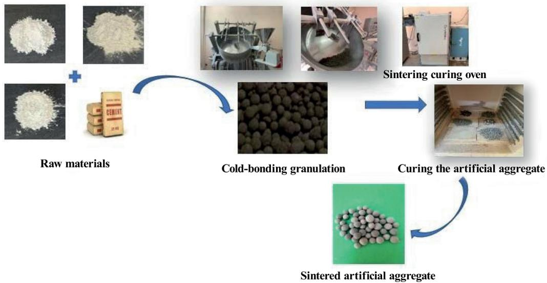
Fig. 4 Sintering manufacturing process
