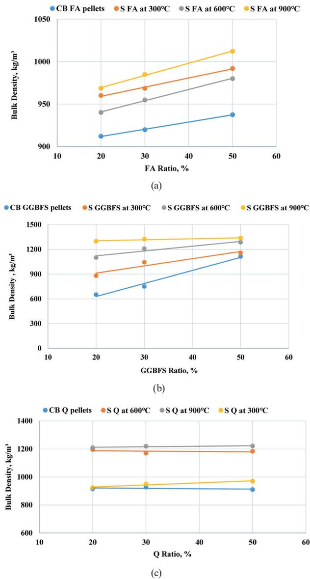
Fig. 8 Bulk density of (a) FA, (b) GGBFS, and (c) Q aggregates at the cold-bonded and sintering methods
