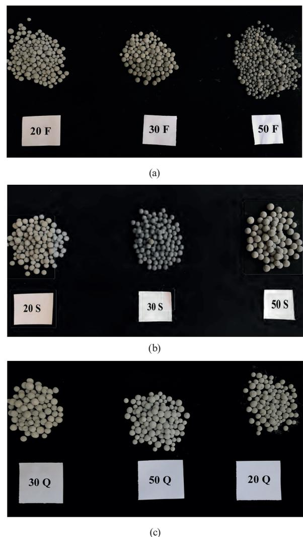
Fig. 3 Photographic view of cold-bonded (a) FA, (b) GGBFS, and (c) Q artificial lightweight aggregates
