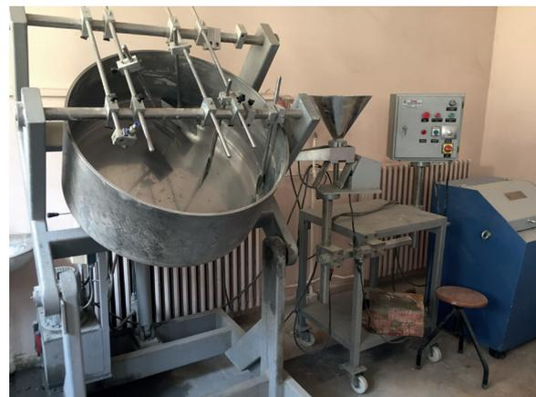
**Fig. 1** Photographic view of pelletization disc
