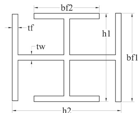
Fig. 10 Welded iHEA column profile
