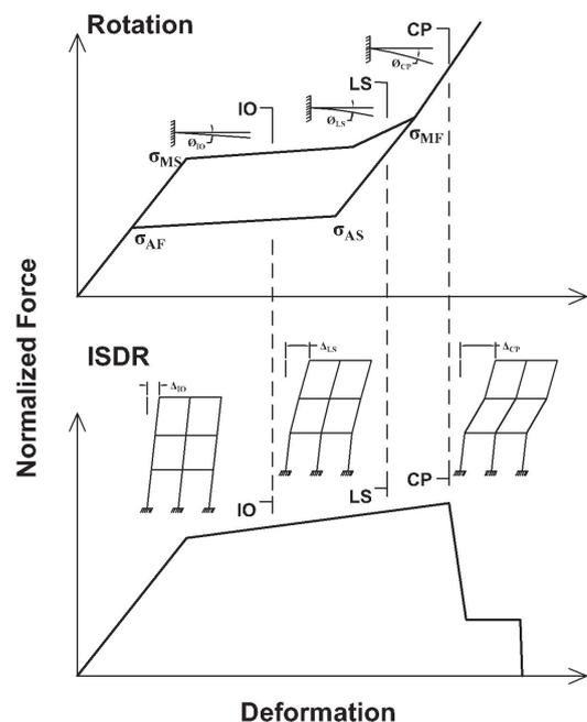
Fig. 4 Performance level of target building, FEMA 356 (bottom) and current study (top)
