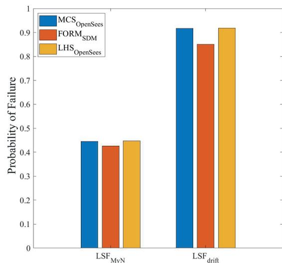
Fig. 6 Probability of failure of MCS vs LHS vs FORM analysis
