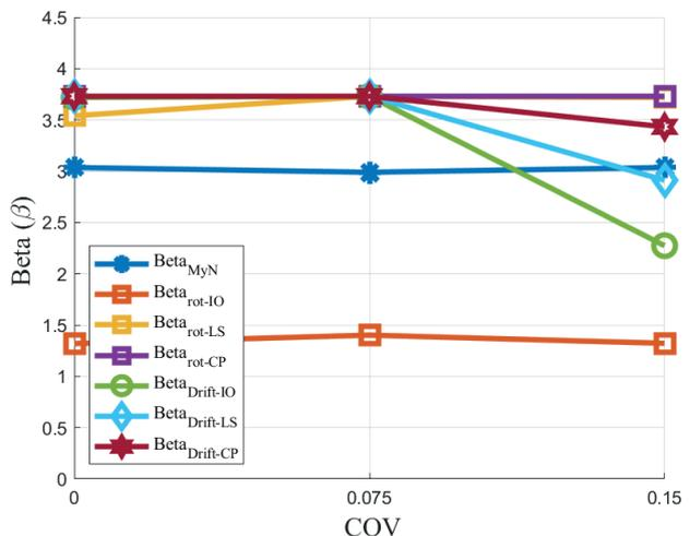
**Fig. 12** Sensitivity of  $\beta$  to material strength ( $F_y$ )
