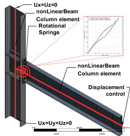
Fig. 8 Fully detailed FEM connection configuration and simplified model (red color)
