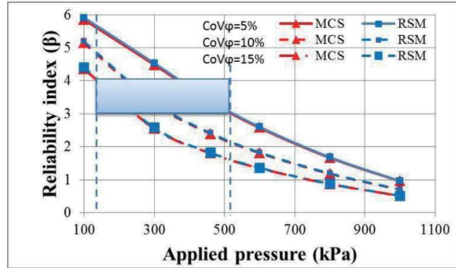
Fig. 6 Results of the reliability analysis using RSM-CCD model and MCS, versus applied pressure for different  $CoV\phi$  ( $\mu_\phi = 33^\circ$ ;  $\mu_\gamma = 15.8$  kN/m<sup>3</sup> –  $CoV\gamma = 10\%$ ;  $\mu_c = 12$  kPa –  $CoVc = 30\%$ ;  $CoVq = 20\%$ )
