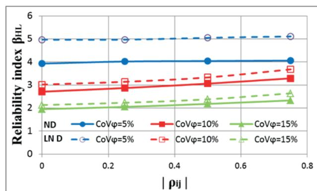
Fig. 4 Reliability index of ultimate bearing capacity for normal (ND) and lognormal (LND) distributions of input soil variables ( $\mu_\phi = 33^\circ - \text{CoV}\phi = 5-15\%; \mu_\gamma = 15.8 \text{ kN/m}^3 - \text{CoV}\gamma = 10\%; \mu_c = 12 \text{ kPa} - \text{CoV}c = 30\%$ )
