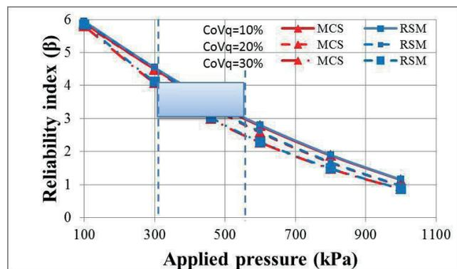
Fig. 7 Results of the reliability analysis using RSM-CCD model and MCS, versus applied pressure for different  $CoVq$  ( $\mu_\phi = 33^\circ$  –  $CoV\phi = 5\%$ ;  $\mu_\gamma = 15.8$  kN/m<sup>3</sup> –  $CoV\gamma = 10\%$ ;  $\mu_c = 12$  kPa –  $CoVc = 30\%$ )
