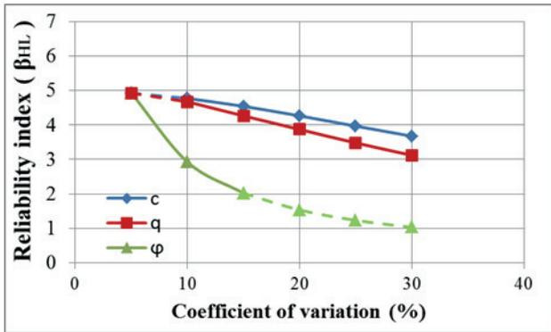
Fig. 5 Reliability index versus different levels of uncertainties using normal distribution ( $\mu_\phi = 33^\circ$ ,  $\mu_c = 12$  kPa,  $\mu_q = 460$  kPa)
