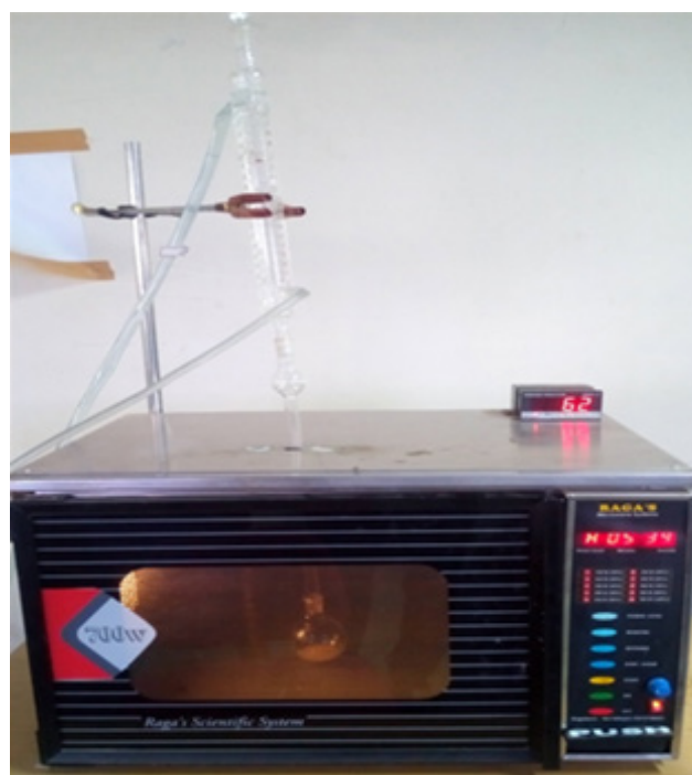
Fig. 1 Experimental setup for microwave synthesis of AOME
